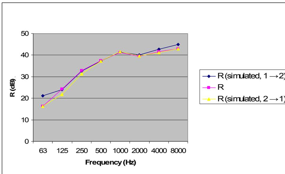
Figure 6. The simulated sound reduction index; results from two different directions of sound transmission; for comparison the calculated resulting reduction index from Table 5 is also shown
