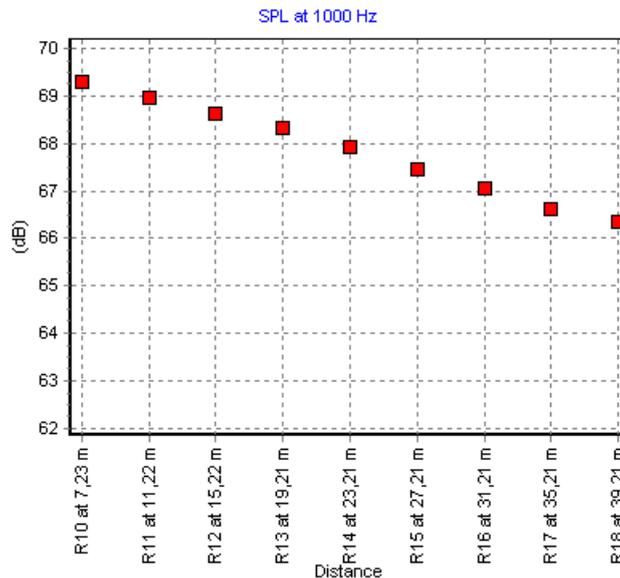
Figure 3. The sound pressure levels in nine positions covering the length of the 40 m long receiver room
