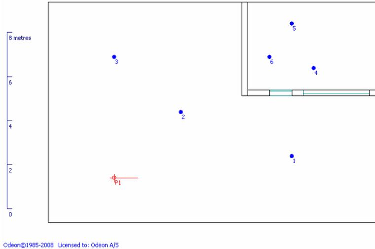
Figure 5. Plan of the test example indication positions of source in the hall and six microphone positions.
