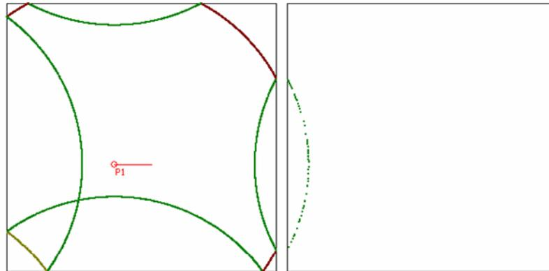
Figure 1. Illustration of a sound wave being reflected from the boundaries in the source room (left) and partly transmitted into the adjacent room. P1 is the source.
