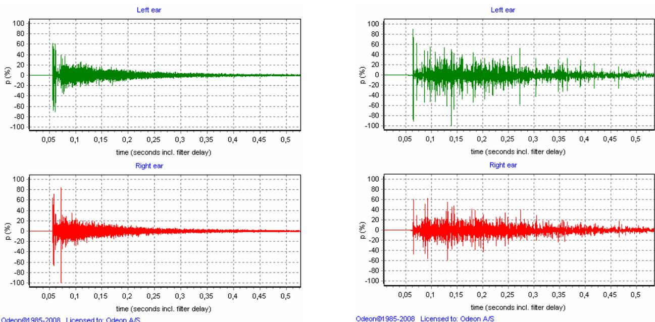
Figure 7. Calculated binaural room impulse responses from the example in section 3 with sound source in the hall; left: position 1 in the hall; right: position 4 in the office. Only the first approx. 0.5 s is shown.
